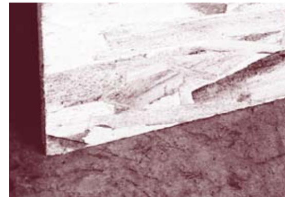
Chip board or OSB is made of wood chips and glue.
